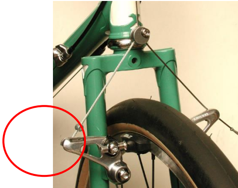
Places to check that your brakes are attached on two kinds of bicycle brakes
